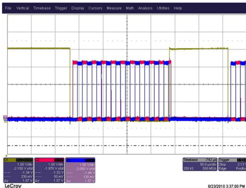
Slika 6.15: Modulirana signala REPORT1_A in REPORT2_A s frekvenco 50 kHz
