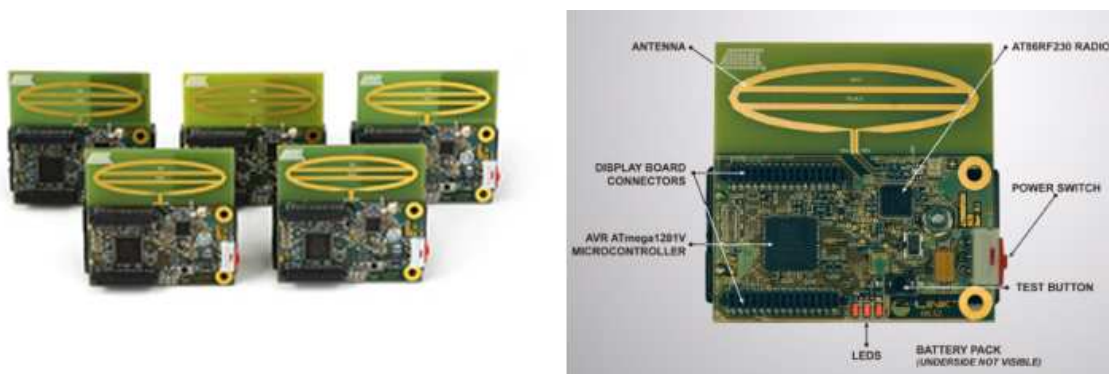
Slika 6 – Atmel® AVR® Z-Link™ ATAVRRZ200 Development kit proizvajalca Atmel
